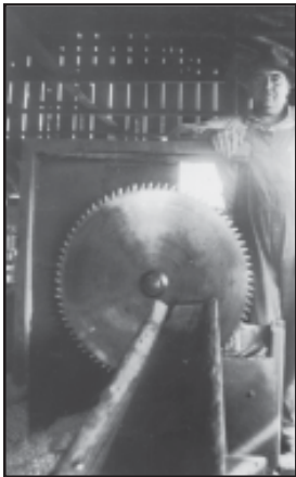
Joe Ware, in 1935, by vertical cut off saw used to square off ends of logs prior to sawing. Trough where log was placed is in foreground. (Photo courtesy of Nelson Ware)
